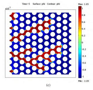
**Figure 3**. Stable drainage flow at M=0.1 in uniform anisotropic medium (a); unstable drainage flow at M=300 (viscous limit) (b); same case as (b) at capillary limit (c).
