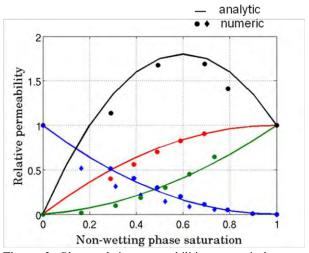
**Figure 2.** Phase relative permeabilities: numerical (symbols) and analytical (solid lines) results for wetting (blue) and non-wetting phase at *M*=0.1 (green); 1 (red); 10 (black).
