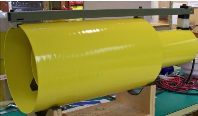
The carbon-fiber variant of doubly resonant sound source
