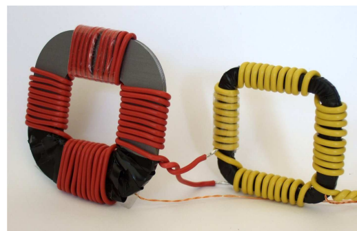
Figure 1. Transformers with laminated soft magnetic ring core for static and dynamic hysteresis measurements.
