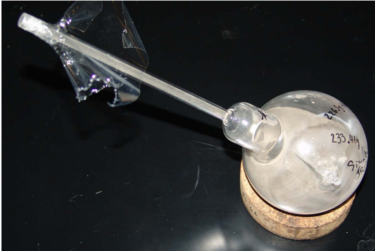
Fused silica vessel with lunar permafrost simulant.
