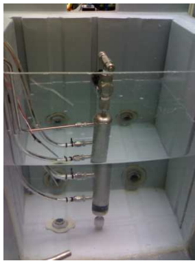
Figure 3. Experimental apparatus: reactor into the water bath.
