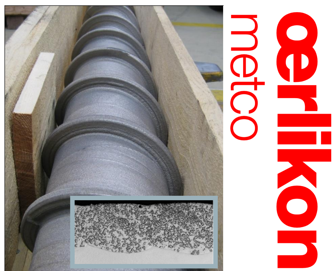
Figure 2. MMC coating on conveyor screw (courtesy of Oerlikon Metco)
