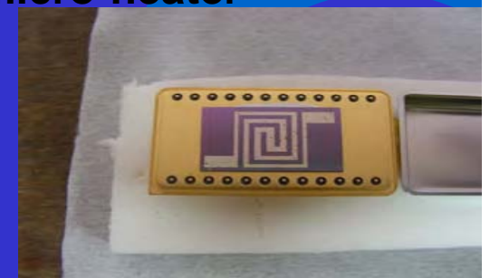
Photograph of Gold wire bonded, packed micro-heater
