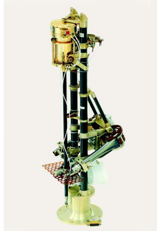
Figure 2. MUPUS experiment aboard the Rosetta comet lander Philae .
