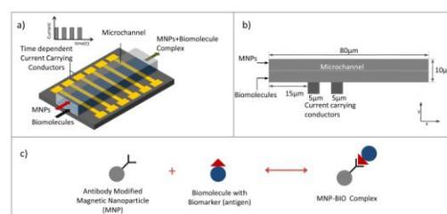
**Figure 1.** Schematic of time dependent magnetic tagging process: a) a three-dimensional conceptual representation of the microfluidic system, b) a 2D cross-sectional view used to develop finite element COMSOL model, and c) binding reaction between MNPs and biomolecule using antigen-antibody chemistry.
