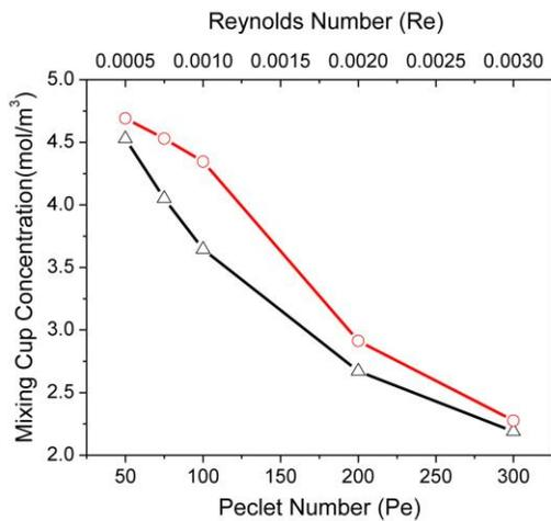
**Figure 3.** Mixing cup concentration variation with Peclet and Reynolds Number, red line with circle is when magnetic actuation was used whereas, black line with triangle is for no magnetic actuation scenario.
