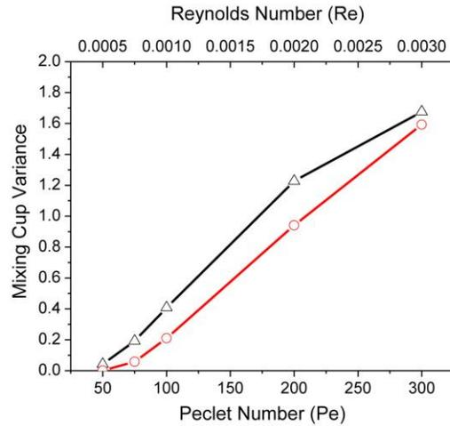
**Figure 3.** Mixing cup variance variation with Peclet and Reynolds Number, red line with circle is when magnetic actuation was used whereas, black line with triangle is for no magnetic actuation scenario.
