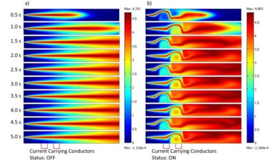
**Figure 2.** Concentration Profile of MNP tagged biomolecule complex formed during the bulk phase reaction taken at different times with microchannel. (a) no magnetic actuation, and (b) time-dependent magnetic actuation
