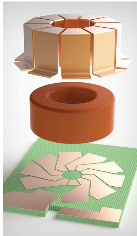
Figure 2. Exploded view of the hybrid winding concept for a toroidal inductor.
