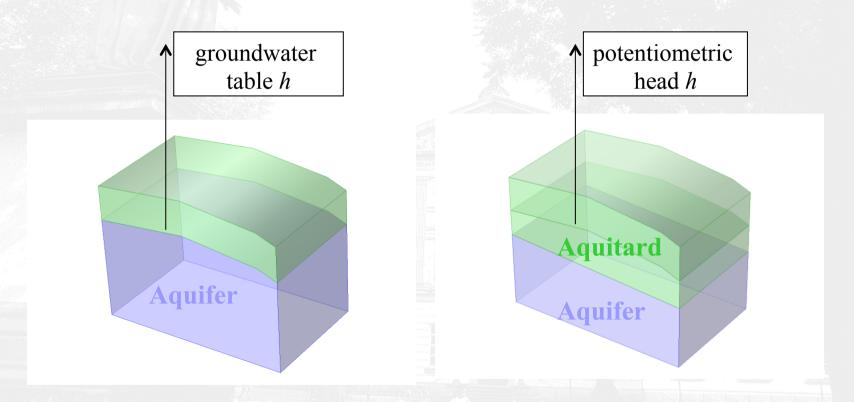
An **aquifer** is an underground layer of water-bearing permeable porous unconsolidated materials
