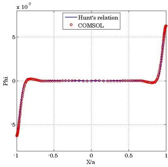
**Figure 2:** Comparison of Non-dimensional electric potential across the side walls
