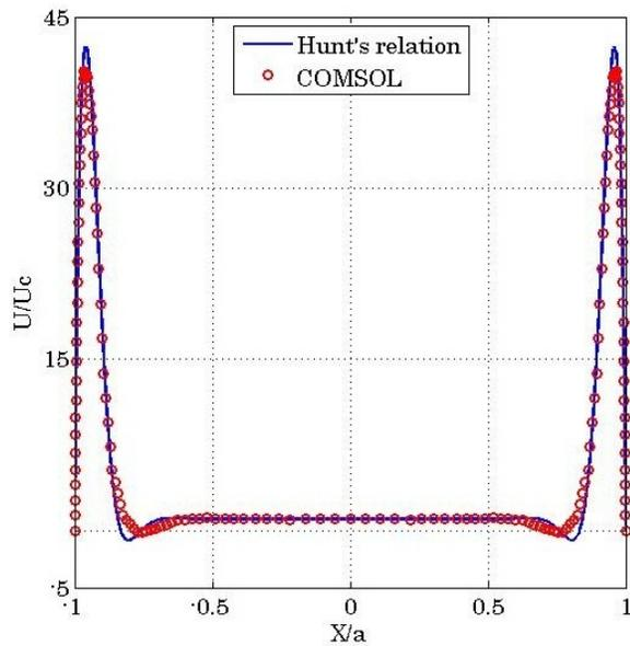
**Figure 1:** Comparison of Non-dimensional velocity across the side wall. Formation of velocity jet near the side wall boundary layer could be nicely captured.
