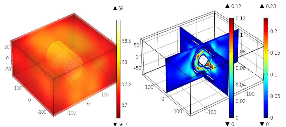
**Figure 3.** Temperature and velocity. Stationary solution.  $V_0=80\text{kV}$ ,  $Q_0=150\text{W}$ . Dielectric cylinder  $\epsilon_r=2.3$ .
