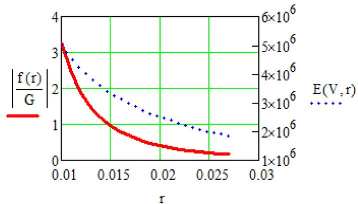
**Figure 1.** Ratio of electric force to specific gravity ( $G=8.83 \cdot 10^3 \text{ N/m}^3$ ) in oil between coaxial cylinders (red) and field  $E$  [V/m] for  $r_{in}=1\text{cm}$ ,  $R_{out}=2.72\text{cm}$ ,  $\epsilon_r = 2.3$ , and  $V=50\text{kV}$ .
