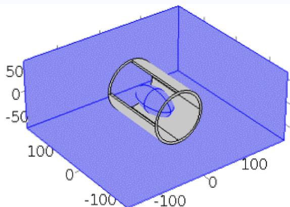
**Figure 2.** Metal vessel filled by transformer oil. Heat  $Q_0$  is generated by ellipsoid sitting at a high potential  $V_0$ . Optional dielectric cylindrical shell. Vessel cooled by natural convection and radiation.
