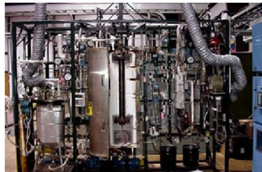
Figure 1. Pilot Unit from University of Tulsa Delayed Coking Project, showing the coke drum and the furnace in the bottom.
