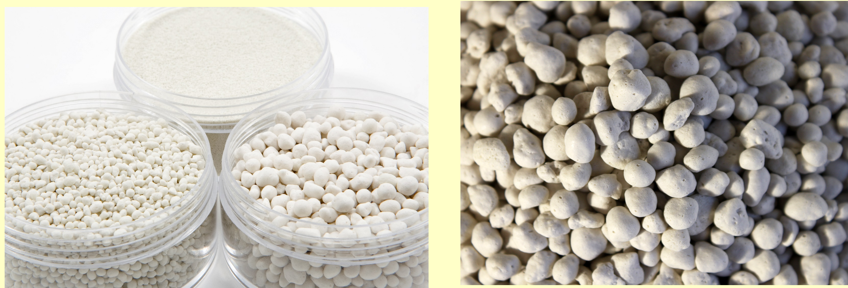
Figure 1. Porous glass - Poraver®
