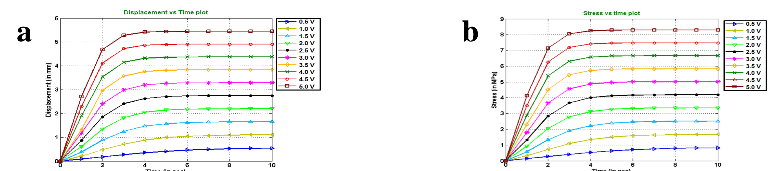
Figure 3: Transient analysis of IPMC actuator shows: (a) Displacement and, (b) Stress variation with time for various applied voltage.
