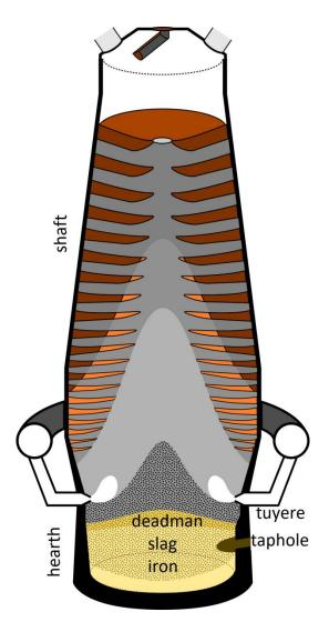
The blast furnace is a type of counter current shaft furnace used for iron ore reduction and smelting to produce industrial liquid iron.
