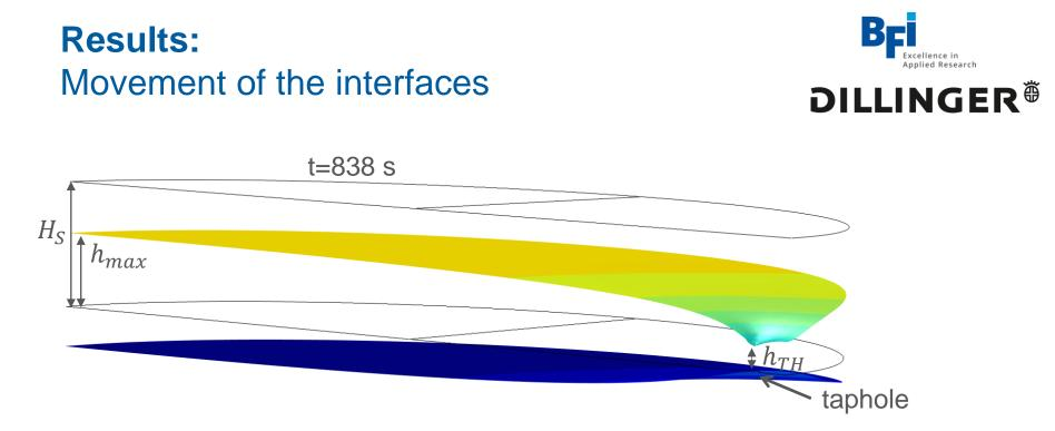
Typical shape of the slag/gas and slag/iron interface at the end of tapping
