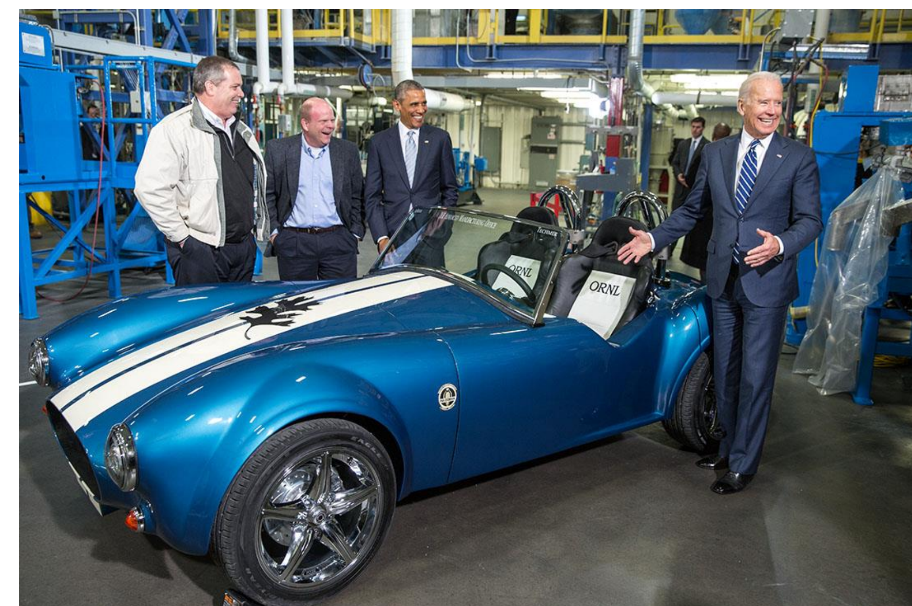
3D printed Shelby Cobra at ORNL
